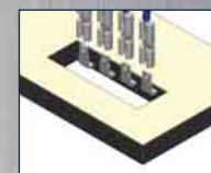
Faston tabs from inside the bus bar, saves space!
