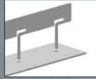
Ring lug terminations using cinch stud hardware in formed tabs.
