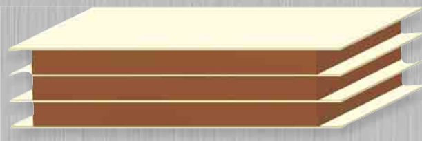
Open Laminated Construction
